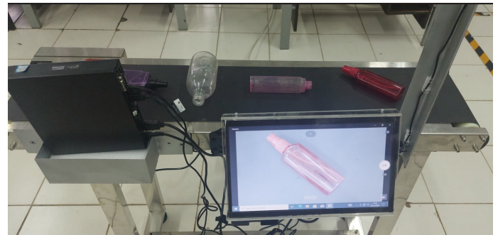
Figure 1. Capturing the Digital Images of Plastic Waste
