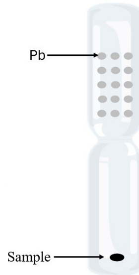
Figure 2. Quartz Model as a Corrosion Test Vessel for Samples in a Pb Environment
