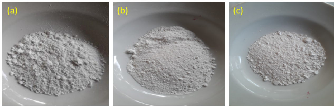
Figure 3. Results of \text{TiO}_2/\text{CaTiO}_3 Synthesis with Variations in Calcination Temperature (a) 700^\circ\text{C} (b) 800^\circ\text{C} and (c) 900^\circ\text{C}
