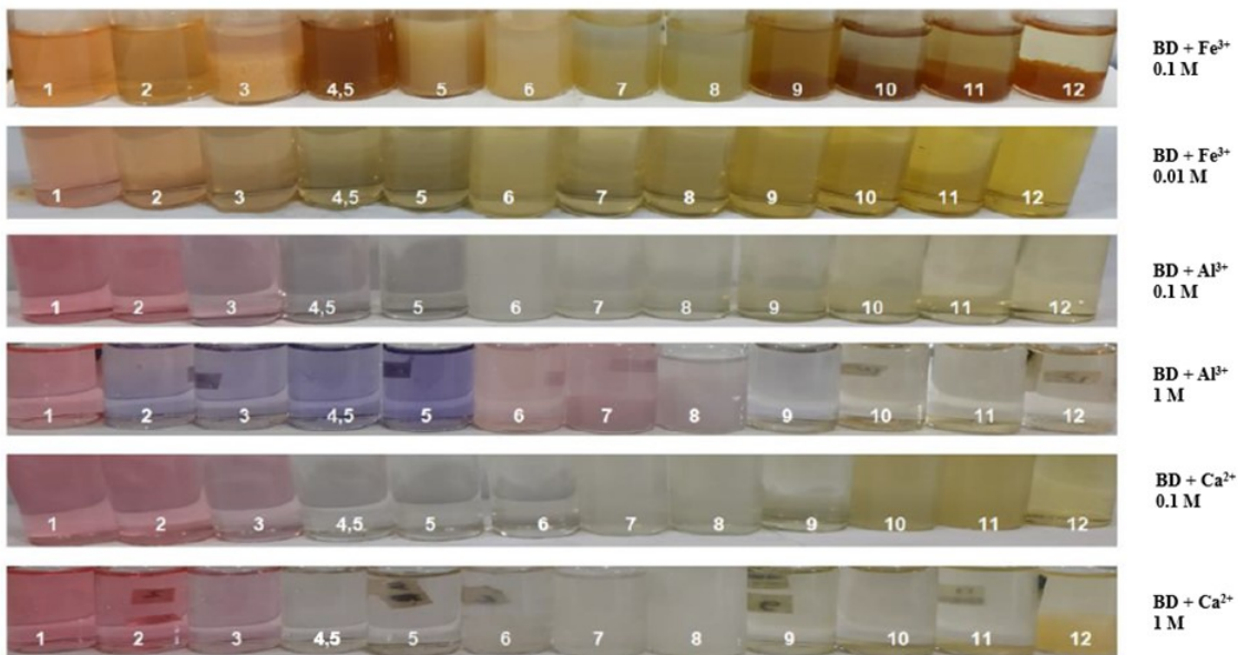
Figure 5. Colour Stability of Anthocyanin-Metal Complexes at pH 1-12 with Different Concentrations. BD: Java Plum fruit Extracts
