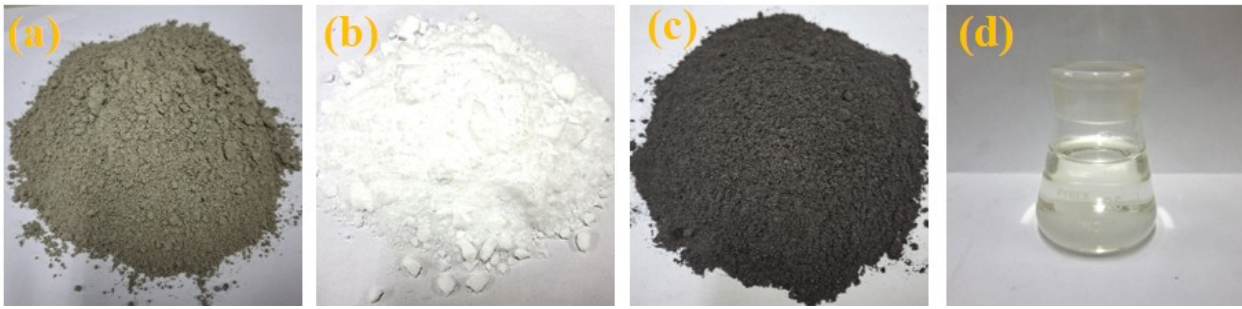
Figure 2. (a) Ordinary Portland Cement (OPC), (b) Nano Silica ( nSiO_2 ), (c) Palm Oil Boiler Ash (POBA), (d) Polycarboxylate Superplasticizer (PCE)
