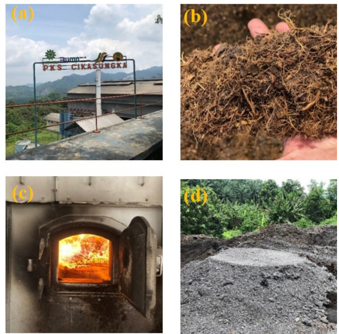
Figure 1. (a) Palm Oil Mill (PKS) Cikasungka (b) Shell and Fine Fiber (c) Combustion Process, (d) Oil Palm Boiler Ash (POBA)
